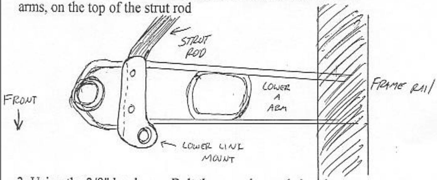
3. Using the 3/8" hardware, Bolt the sway bar and chassis mounts to the frame. Then bolt the end links through the sway bar to the end link mounts. Lightly snug the bushings. Lower the vehicle to the ground & drive it back & forth to settle the suspension. Reach under & tighten the end links.
