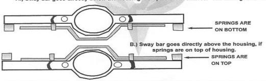
3. Position arms parallel with the springs. Assemble end links straight up to chassis mount, drill hoes and bolt in place. Place mount to keep bar even with springs.
