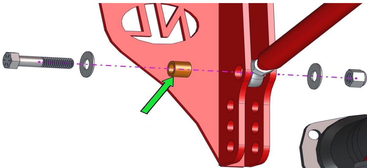
using the Frame Mounting Bracket Spacer and **1/2"-13** Hardware. Do not tighten the bolt for the next step.
