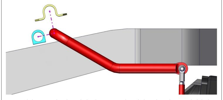
With the Sway Bar loosely attached to the Sway Bar Link, set the bar to be 90 degrees to the link. The
