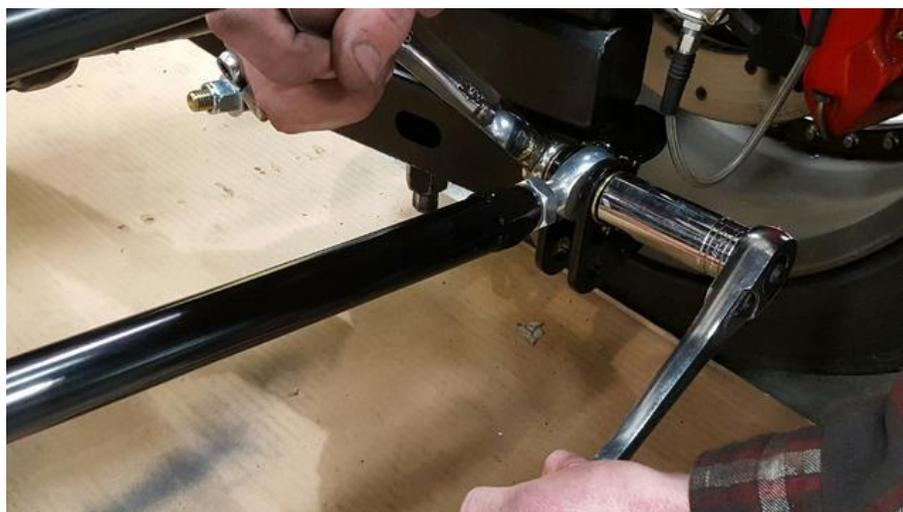
Now you can prep the shocks. Bearing mounted coil-overs often need the bearings installed. You will need some snap ring pliers and Loctite. (red or blue is OK) Install one snap ring, then coat the bearing outer surface with Loctite. I like to coat the bearings and let them sit a while. 10 minutes is good. Slide the bearing in place and put in the second snap ring. Install the other bearings the same way.
