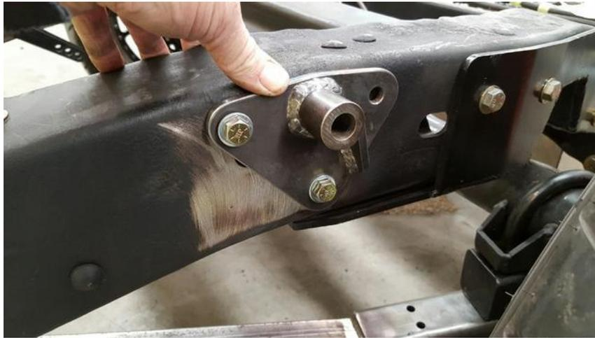
Now it's drill time. Use a 3/8" drill to drill out the rear hole for mounting the coil-over bracket. Then use a 5/8" bit to drill through the frame for the upper coil-over mount bolt. Put the third mount bolt in place.
