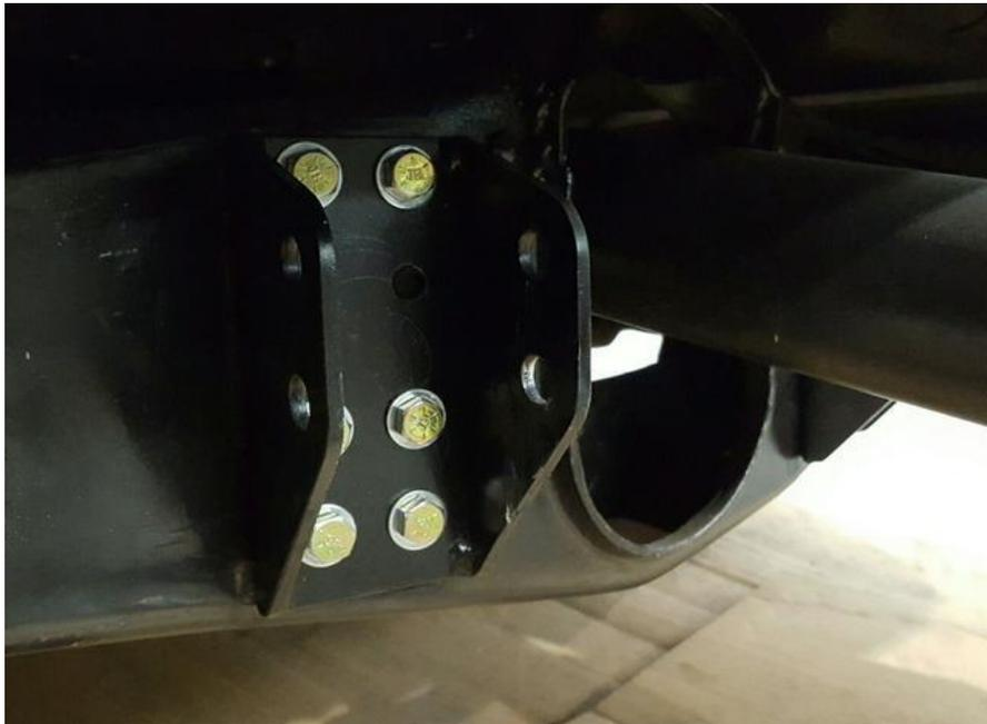
**The new trailing arms go in next. The trailing arms are adjustable in length. This adjustment is used to set the wheelbase and to square the axle in the chassis. In the long run you may drop the arms a few times to get it perfect. No big deal, it's like carb jetting, with really big parts. The arms bolt in just like stock with new hardware provided up front. Use anti-seize on the threads, and the OE U-bolts for mounting the axle.**
