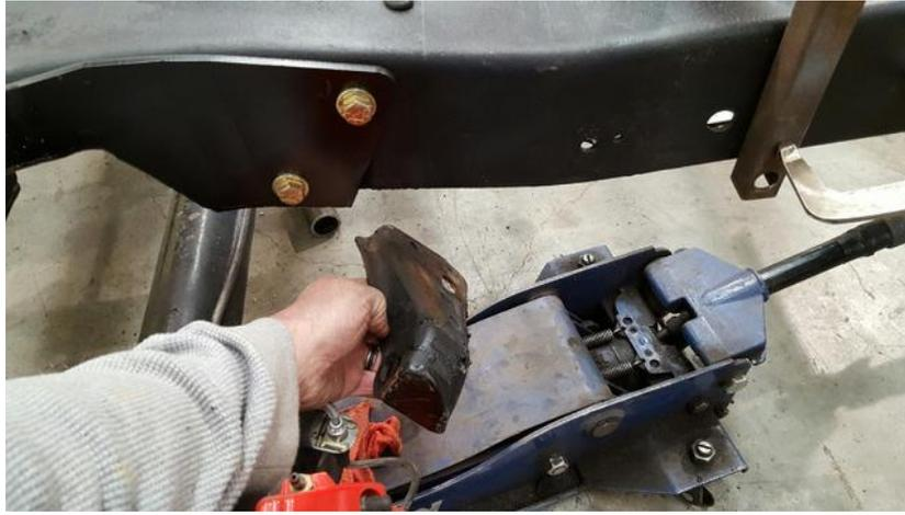
**The new Panhard mount uses this hole to locate it. Chase it with the 3/8" drill bit and bolt the new bracket in place. There are two mounting rails for the panhard rod on the inside of the bracket. They should be at 90 degrees to the frame rail flats. Or, if the truck is level front to back, these mount rails should be straight up and down. Notice that the bracket fits the frame profile nicely when it is in it's proper location.**
