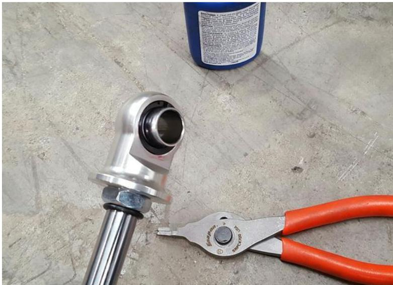
**Next, go get some anti-seize. Not grease or oil , go get some anti-seize. Coat the top 3" or so of the shock threads. You can clean up the excess later, but doing this will make ride height adjustments a LOT easier. Then assemble the springs and adjusters onto the shocks.**
