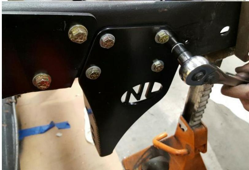
**There is only one hole left to drill. This is for the panhard bracket brace. To get the roll center low, really low, compared to a stock or modified C10, the mounting brackets have to drop down pretty far.**
