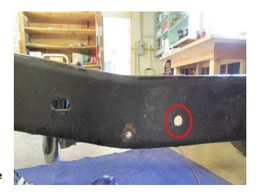
• If your frame rail is missing this hole the Frame Shock Mounts can be positioned by drilling a 5/8" hole at **17 5/16**" from the end of the frame rail, and **1**  $\frac{3}{4}$ " from the bottom of the rear frame section.
