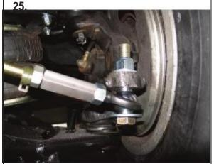
25. Using the 5/8" grade 8 bolts, washers, and nylock nuts, bolt the rod ends to the spindle as shown. Tighten to 100ft lbs.
