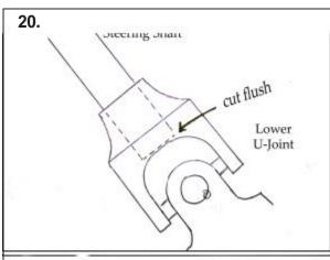
**20**.Cut the shaft so that it fits flush inside the lower u-joint on the bottom side.
