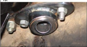
**15.** Use the 5/16" bolts, nuts, and washers to bolt the bearing mount to the underside of the frame rail.
