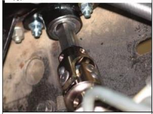
18. Slide the 3/4 - 36 spline u-joint onto the rack.
