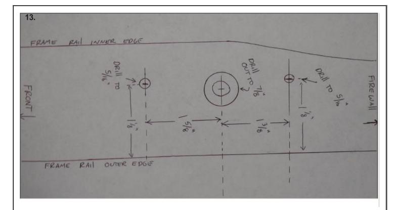
**13.** Ahhhh!! Got that out of your system? Good. Pay attention now. We assume (hate that, but we had to) that the motor is using the back two holes (most are). There are three holes in the top of the frame. If the mounts are in the 'front' and 'center' holes, you will need to move them, and if there is a 4" gap between the motor and the firewall, you really need to consider moving it back. Otherwise, all the work spent upgrading the steering is sort of like putting lipstick on a pig.
