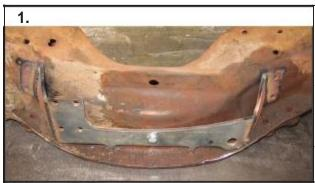
1. Here is a picture of the rack mounting plate on a stock C-10 crossmember. This is a front-steer set up. Yes, you can do this with the motor in place, as well as all the suspension. Start by removing the steering box, idler arm, and steering linkage. Keep the steering shaft for later.
