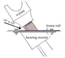
**19**. You will need to cut the steering shaft. When installed, you want 1/8" to 1/4" of clearance between the u-joint and the frame rail on the top.
