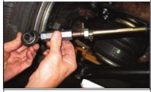
24. The tie rod end on the rack is metric. Put the metric jam nut on first. Thread the rod end, with jam nut on, into the adjuster so that only 1/4" of the thread is showing in the rod end.
