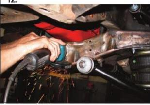
**12**.Use a grinder to cut the lip back for clearance. Repeat Step # 11. Until it clears.
