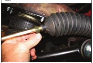
**23**. It helps to pull the spring clamp off the end of the rack boot. This makes it easier to adjust.
