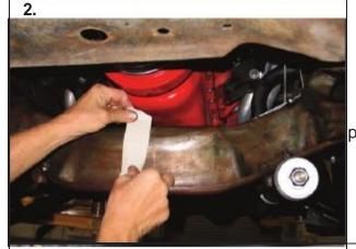
2. Once you have cleaned the crossmember, put a piece of masking tape on the front face, in the center
