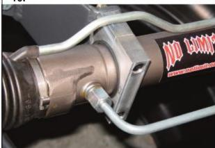
10. Assemble the billet clamp as shown.Yes, you can cut the rubber isolator if you must.You may need to use the 5/16" drill bit to clean the holes in the bracket.Once this is snug, then tighten all 3 rack mounting bolts.
