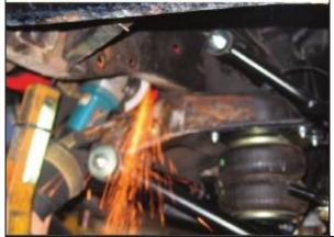
17. Grind the bottom edge of the rail for clearance.
