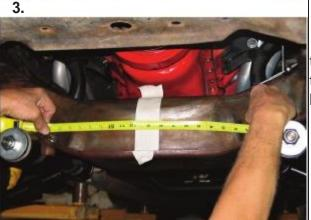
3. Using a tape measure, find and mark the center of the crossmember. You can use the framerails, and/or the u-bolts for the lower a-arms. Be accurate, and double check.
