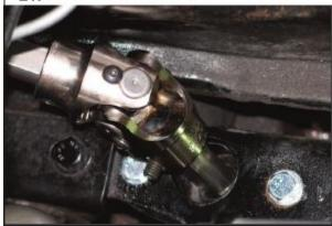
21. Sand and debur the cut shaft.
