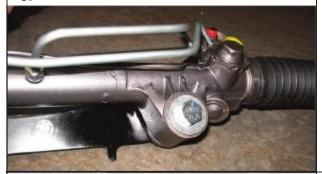
9. Mount the rack to the bracket. Use the 5/8" bolt, nut, and washers on the driver's side-- Finger tight only. Then......
