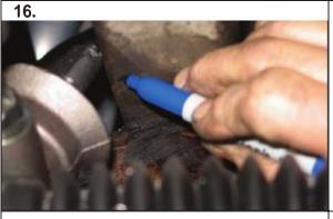
16. Oops - - You need to check one more thing. With the rack held in place, mark for clearance between the rack (with the steering u-joint in mind) and the frame.
