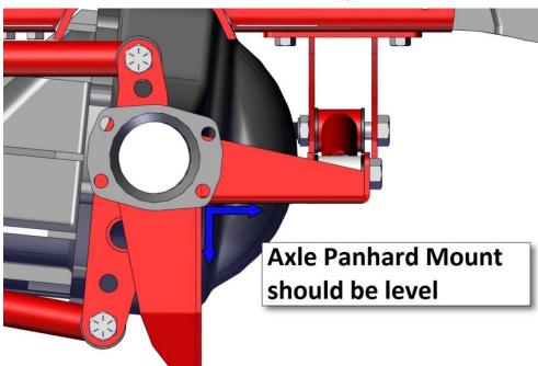
• With every thing tacked into position, carefully remove the axle not to break any tack welds, if any break resetting the axle will be necessary in order to have a correct alignment. Set the axle onto a secure surface and finish welding the brackets. (Note: for best results weld in increments of 1 inch to 1 ½" inches and then switch sides repetitively to prevent any brackets or the tubes from warping).
