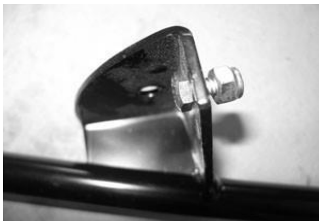
2 - 1/4-20 x 1/2 are provided for hood braces to act as a stop
