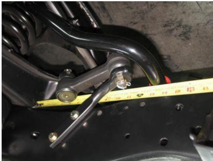
3. Put the red urethane mount bushings around the sway bar, on the straight center section, appx. 3" from the bend on each side.
