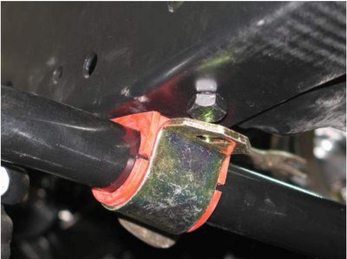
1963 – 1972. You will need to drill two holes on each frame rail. From the underside of the frame, measure from the suspension crossmember forward and mark for the two holes at 12" and 15". Drill the holes in the center of the rail (side to side) Use an 1/8" bit to drill a pilot hole, and then drill the hole out to 3/8".
