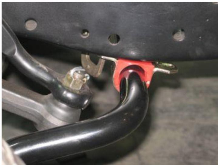
Bolt the sway bar and mounts to the chassis with 4 3/8" x 1 1/4" bolts, 8 sae flat washers and 4 nylock nuts. The sway bar fits over the steering linkage.
