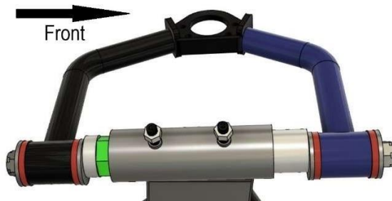
Figure #10: Demonstrates the position of the cam so that it is slid forward thus reducing caster angle.
